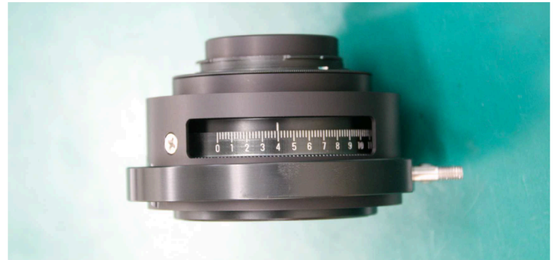
Figure 5 Side view of lens assembly (Indicator read of helicoid is set to be “4” in the photo)
