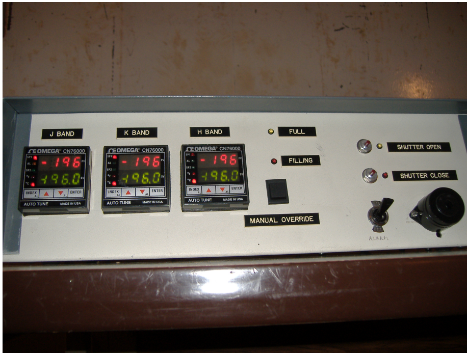
Figure 8: Focal Plane Array temperature controller.
